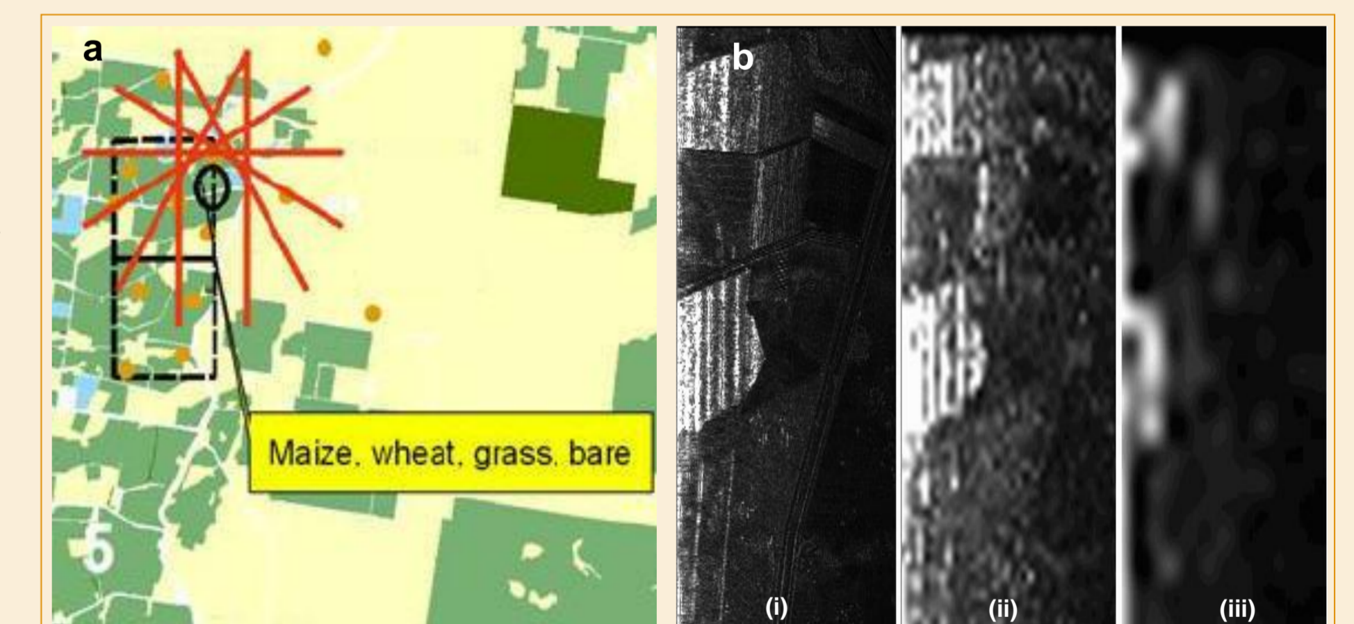
Fig. 4: a: Overview of multi-azimuth flight lines (in red) and coverage (black circle) in Area 1; b: Spatial scaling of radar backscatter: (i) original data observed at 10m resolution; (ii) data scaled to 50m resolution; and (iii) data scaled to 150m resolution.
